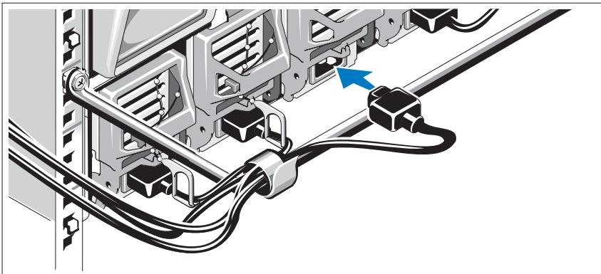
Connect the system's power cables to the system power supplies.
