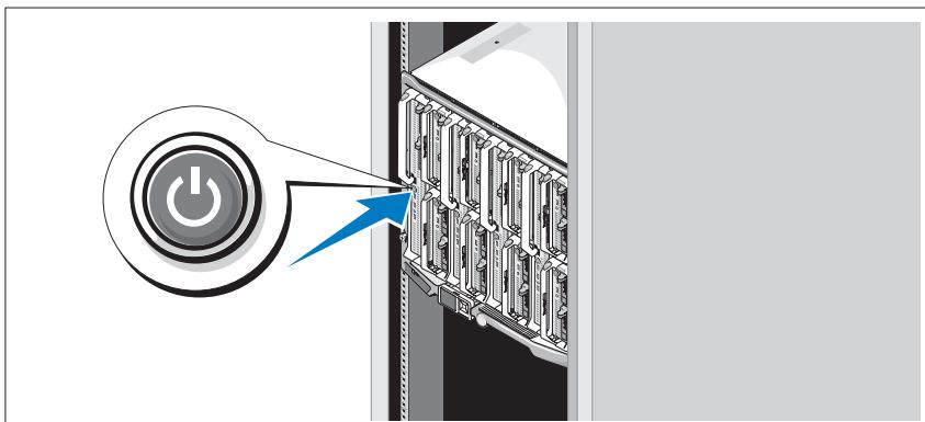
Press the power button on each blade, or power on the blades using the systems management software.
